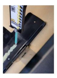
**3.1** First, use the glue gun to pump some glue onto the cardboard, because the mixing ratio is not yet correct.
