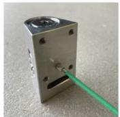
**2.2** Screw the cylinder lock into the lock housing with the adjusting screw until it is secure.
