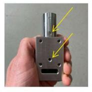
**2.1** Place the cylinder lock in the lock housing as shown in the image above.
