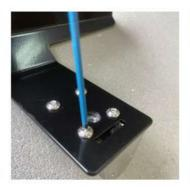
**2.3** Then screw the lock housing to the bracket with the 4 bolts.
