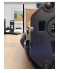
**3.3** Place the battery straight, in the middle of the battery slot on top of the glue. Check carefully that the space on both sides of the battery is equal.
