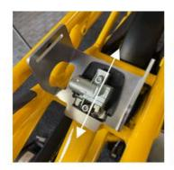
2.1 Place the bracket over the ridge. Put the Bosch lock back in place, but do not fully tighten the screws yet. Place the battery back in the bottom docking and the Bosch lock. Make sure that the Bosch lock clicks properly; if not, you may need to move the lock slightly for proper placement.
