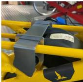
2.2 When the battery clicks properly, slide the pin through the bracket.
