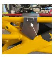
**2.3** Now replace the battery. Stick the supplied piece of foam to the inside of the pin where it contacts the frame. Then slide the pin through the bracket.
