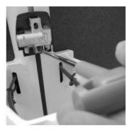
**1.4** Unscrew the two Inbus screws and remove the Bosch lock.
